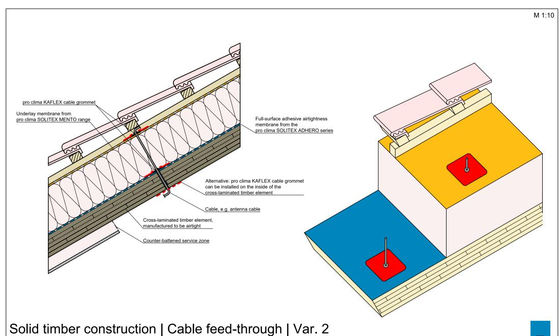
Variant 2: Airtight sealing of the building component with pro clima SOLITEX ADHERO. Airtight cable feed-through with pro clima KAFLEX.
