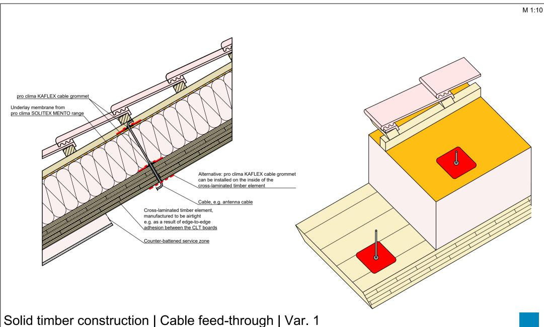
Variant 1: Airtight cable feed-through with pro clima KAFLEX. The cross-laminated timber elements must be manufactured to be airtight.
